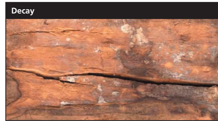
Checking A separation of the fibres along the grain forming a fissure, but not extending through the piece.
