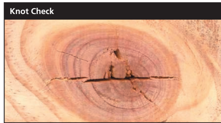
Knot Check A check occurring in a knot.
