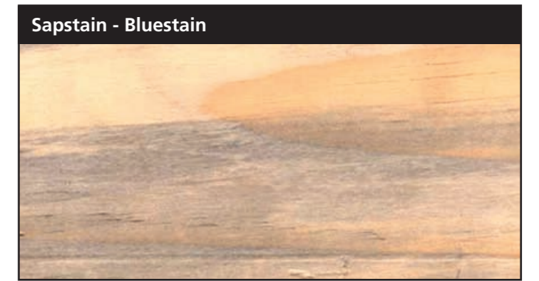
Sapstain - Bluestain A blue / grey discoloration in the timber caused by fungal action, but not associated with decay.
