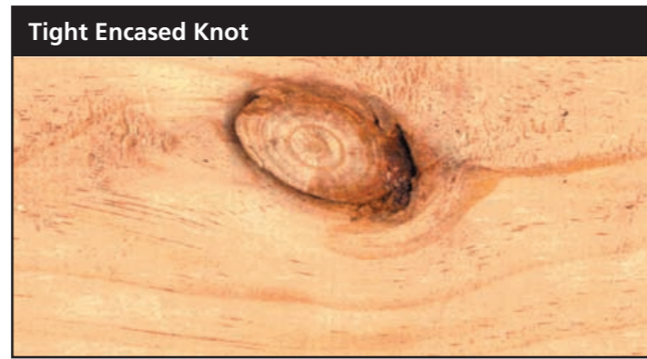
Tight Encased Knot A sound knot in which more than half its perimeter is surrounded by bark, but which is fixed by growth or size so that it will remain in the piece of timber.
