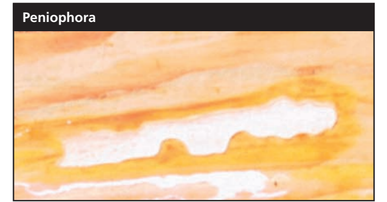
Mycelium Sign of fungal attack on wood affecting strength and potential uses. Easily transferred to non contaminated wood with affected fillets and bearers. Spores can be wind blown.
