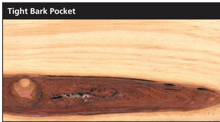
Tight Bark Pocket A bark pocket in which the bark is firmly embedded in the surrounding wood.
