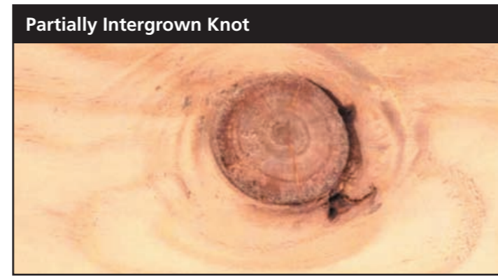
Partially Intergrown Knot A knot that has not more than half its perimeter separated from the surrounding wood by bark.
