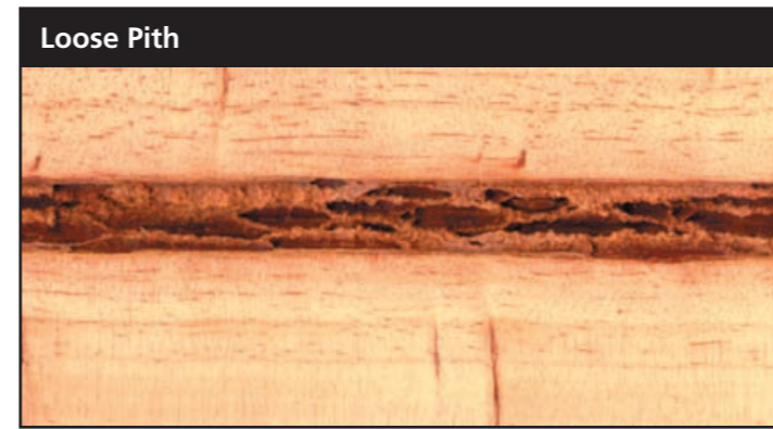
Loose Pith Pith that is generally large in diameter and has many voids in its structure.
